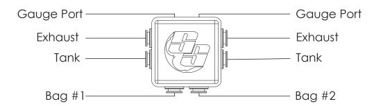
Only one inlet/tank port is required for valve to operate. (See Recommendations below)
