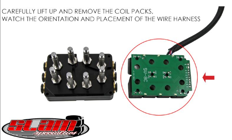
USING A 9/16" SOCKET WRENCH LOOSEN AND REMOVE (8) ARMATURES AND PLUNGERS. BE AWARE OF PLUNGERS AS THEY ARE SPRING LOADED
