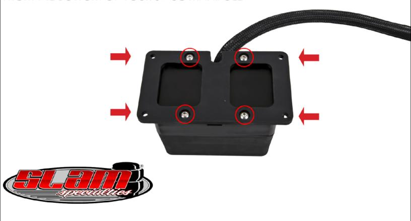
WITH THE (4) #10 SCREWS REMOVED, THE LOWER MOUNTING BASE PLATES CAN BE REMOVED AND SET ASIDE
