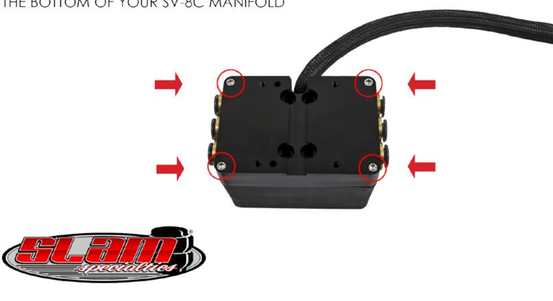
WITH THE (4) #10 SCREWS REMOVED, THE TOP CAP CAN BE CAREFULLY REMOVED AND SET ASIDE
