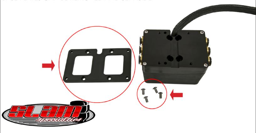
REMOVE (4) #10 SCREWS USING 9/64" ALLEN WRENCH FROM THE BOTTOM OF YOUR SV-8C MANIFOLD
