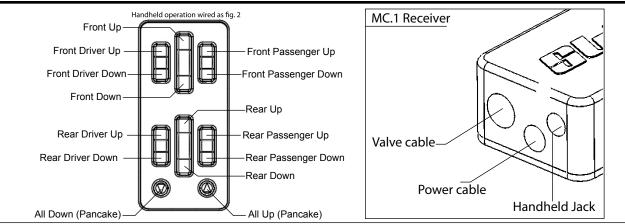
The MC.1 can be wired in multiple configurations depending on the desired orientation of the handheld (fig. 2 and fig. 3). below is the valve wiring diagram for each configuration. Connect the power wire as per fig 1. for **BOTH** configurations. **fig. 1**
