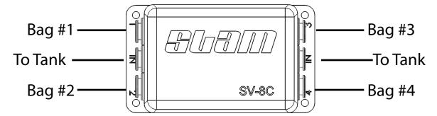
Only one inlet/tank port is required for valve to operate. The second inlet port can be plugged with the included port plug.
