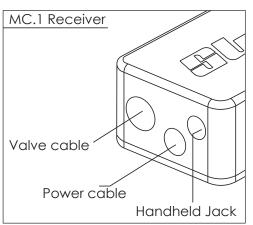
The MC.1 can be wired multiple configurations depending on the desired orientation of the handheld (fig.2 and Fig.3). Below is the valve wiring diagram for each configuration. Connect the power wire as per fig.1 for **BOTH** configurations.
