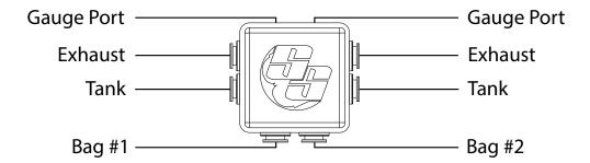
Only one inlet/tank port is required for valve to operate. **See Recommendations below**The second inlet port can be plugged with the included port plug.
